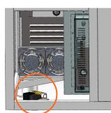
The solenoid valve is shipped attached in the bottom corner of the frame. If using a LSBM, then unscrew the solenoid valve and install it as noted.
